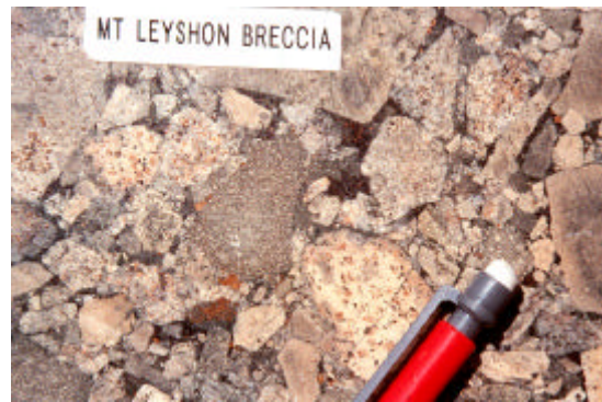
Photo 16. Carbonate-base metal gold mineralization as a breccia matrix, Mt Leyshon.
