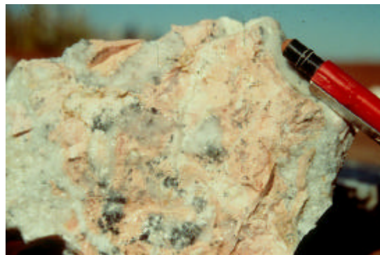
Photo 14. Rio del Medio, El Indio district carbonate-base metal gold mineralization showing rhodochrosite
