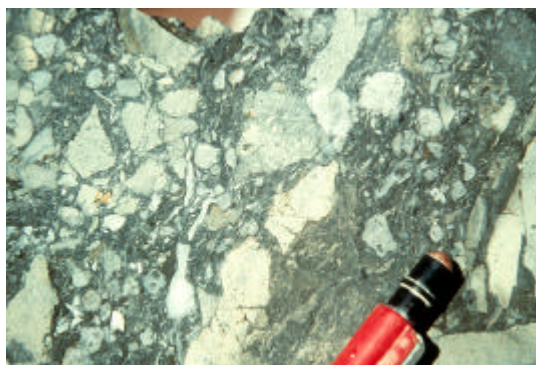
Photo 26. Structurally controlled higher grade replacement sediment hosted gold mineralization, Meikle.
