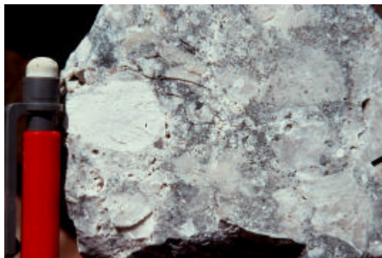
Photo 35. Diatreme breccia with vughy silica altered juvenile intrusion fragment and pervasive silicification of milled breccia, Yanacocha.
