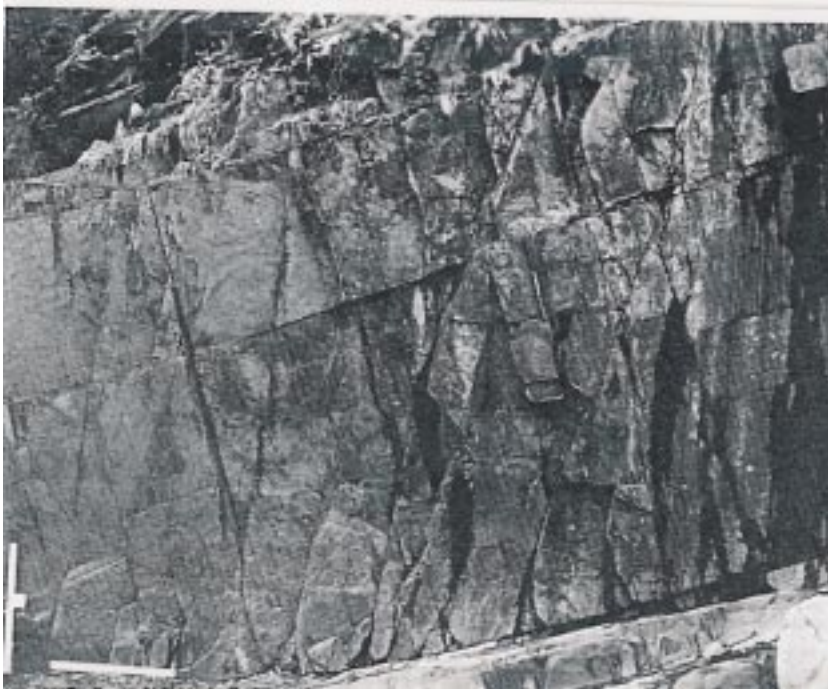
Fig. 5-6 Jointed Ordovician mudstone. The rulers shown are 1 m long (from Hudson and Priest 1979).
